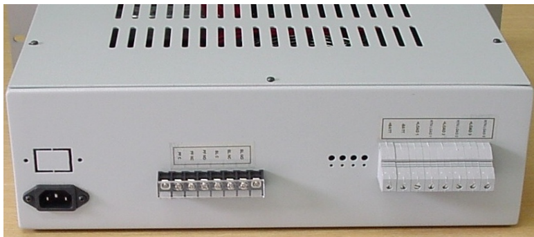
Fig 2: Rear view of a 3U x 19in Rack assembly with High Current Phoenix Connectors
