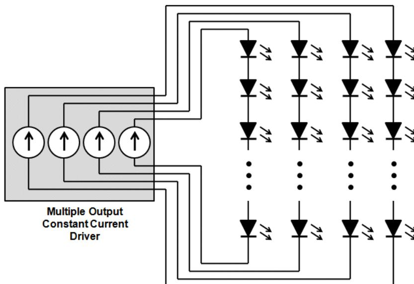
Figure 4. Multi-Channel Configuration
