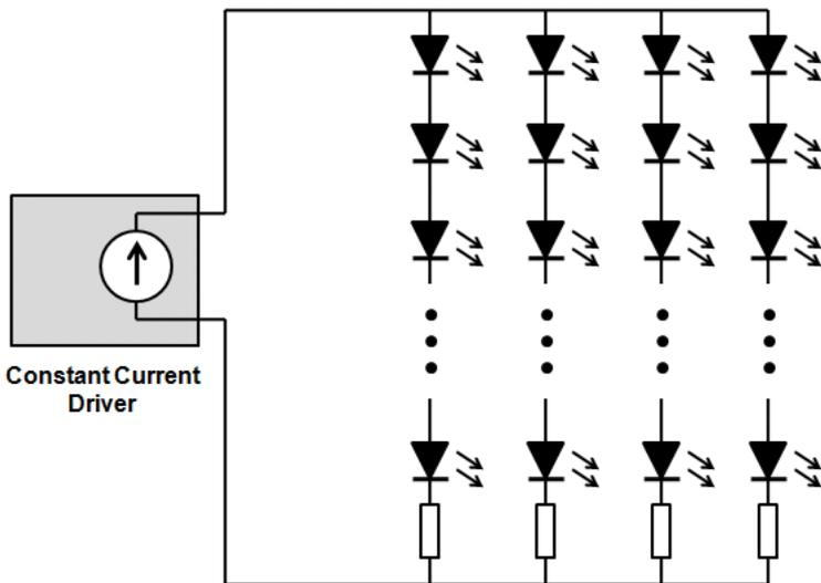
Figure 2. Parallel Strings Configuration
