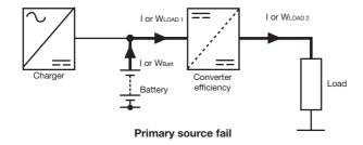
Care should be taken as the load rating on the system may change when the primary source is not available, as this may change the battery Ah capacity required.
