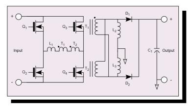
Figure 1.15 - Phase Shifted Full Bridge Converter
