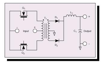
Figure 1.12 - Push-Pull Converter
