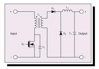
Figure 1.10 - Resonant Reset Forward Converter
