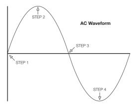
The polarity of the voltage across the wire coils reverses as the opposite poles of the rotating magnet pass by. Connected to a load, this reversing voltage polarity creates a reversing current direction in the circuit.
